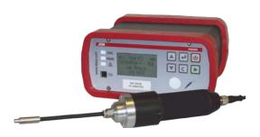
Getting an idea of where the leak is requires a bit more cycle time for air stabilization in the engine, but it can be achieved with a special ATEQ model MF differential flow tester.
